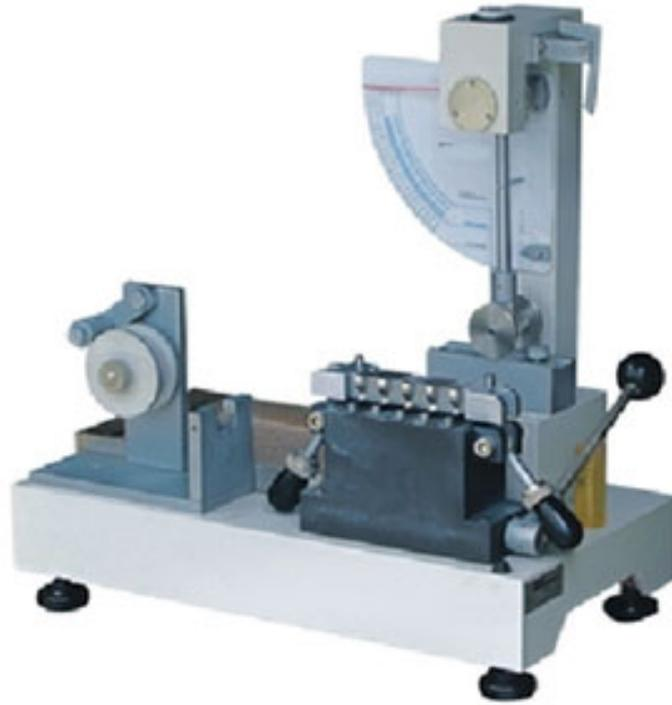
*Fig. 28 (strumento Scott Bond)*
