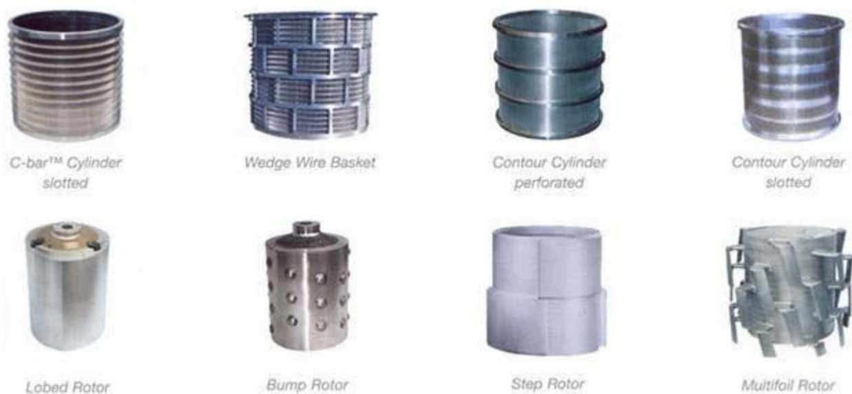
Fig. 5 - Screening: baskets and rotors.
